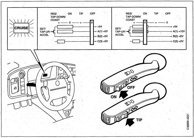
The Cruise Control system is controlled by means of switch 141.
