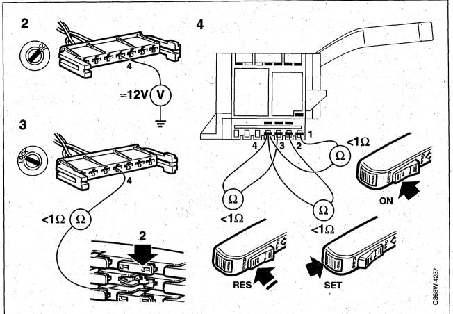
2 If the voltage readings are not OK, check that about 12 V is present across pin 4 of the switch connector and a good ground.
