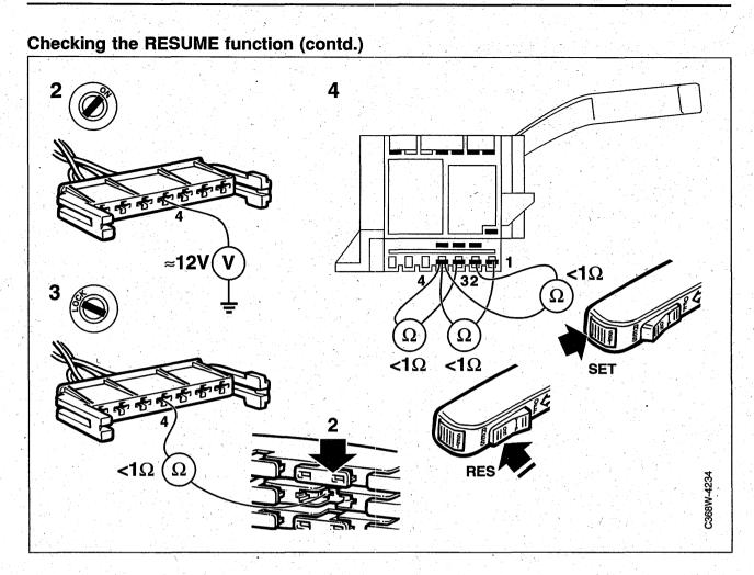
2 If the voltage readings are not OK, check that about 12 V is present across pin 4 of the switch connector and a good ground.
