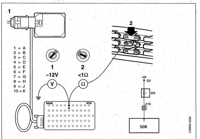
Ignition switch in the LOCK position. Connect a BOB and check the power supply for the Cruise Control system's control module by taking a voltage reading across pin F (6) of the control module connector and a good ground (e.g. a door hinge screw).
