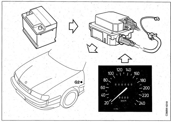
The control module incorporates an electric stepping motor which mechanically regulates the Cruise Control cable connected to the throttle body, either retracting it or extending it according to the speed of the car.
