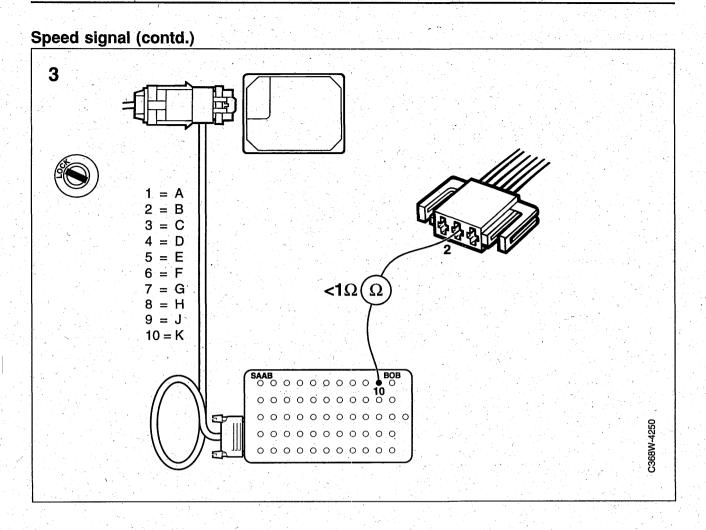
3 If no signal is present, check the wiring.
