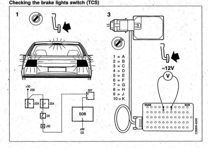
In order for the Cruise Control system to work, at least one of the brake light bulbs must be OK.
