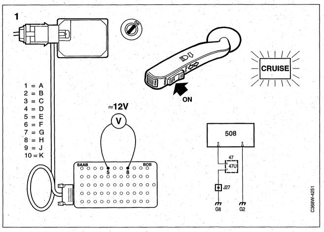
1 Check that about 12 V is present across pin 8 (H) of the Cruise Control connector and a good ground when the Cruise Control system is activated.
