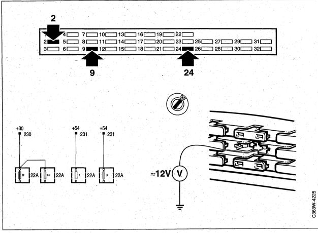
1 Check that the fuse is intact and that a voltage of about 12 V is present on it, as indicated in the table below.
