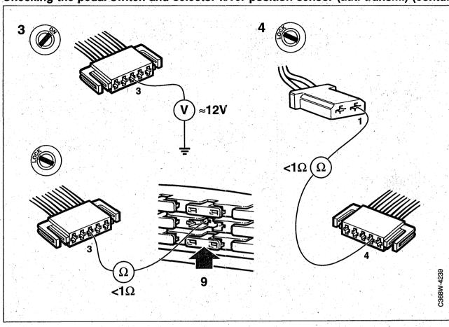
Checking the pedal switch and selector lever position sensor (aut. transm.) (contd.)
