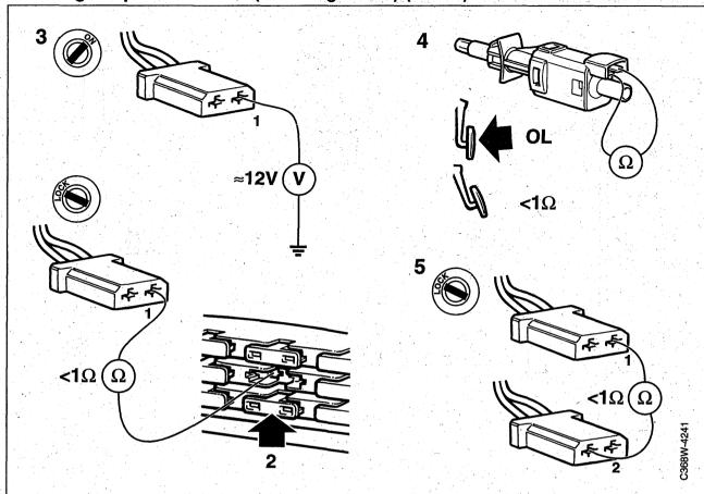
Checking the pedal switches (manual gearbox) (contd.)
