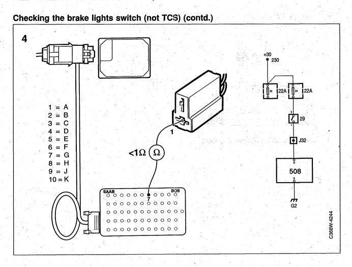
4 If the voltage is not OK, check the wiring for continuity or a short circuit by measuring the resistance across pin 1 of the brake lights switch and pin G (7) of the Cruise Control.
