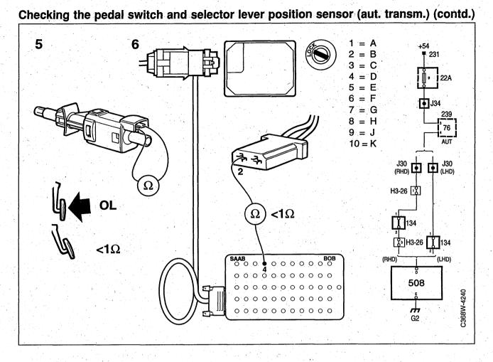
5 Measure the resistance across pins 1 and 2 of the brake pedal switch when the brake pedal is depressed and also when it is not depressed.
