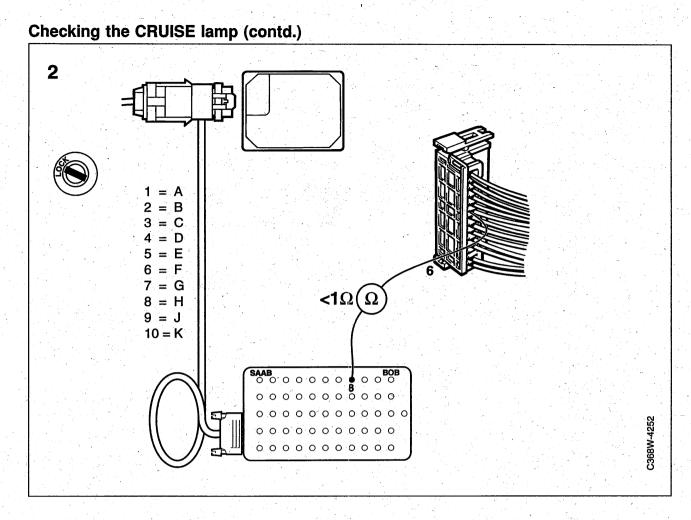
2 If the voltage is OK, check the wiring for continuity or a short circuit by measuring the resistance across pin 8 (H) of the Cruise Control connector and pin 6 of the main instrument display connector.
