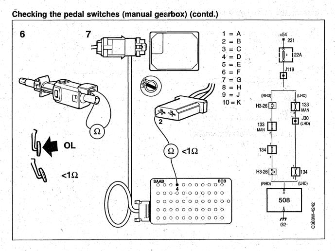
6 Measure the resistance across pins 1 and 2 of the brake pedal switch when the brake pedal is depressed and also when it is not depressed.
