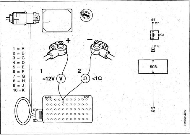
1 Check the grounding of the control module by taking a voltage reading across battery positive and pin E (5) of the control module connector.
