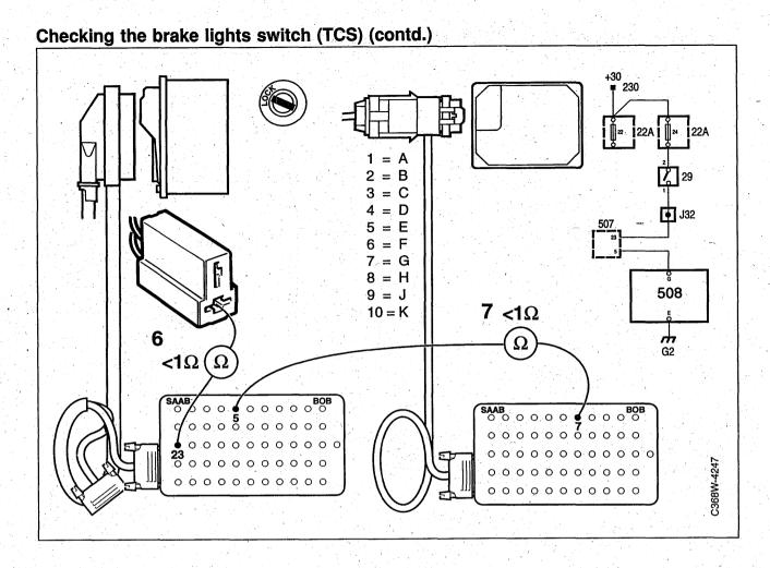
6 Check the wiring for continuity or a short circuit by measuring the resistance across pin 1 of the brake lights switch connector and pin 23 of the TCS control module connector.
