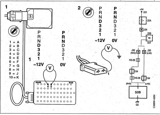
Checking the pedal switch and selector lever position sensor (aut. transmission)
