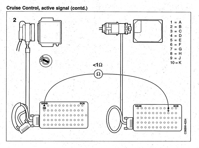
2 Check the wiring for continuity or a short circuit as follows:
