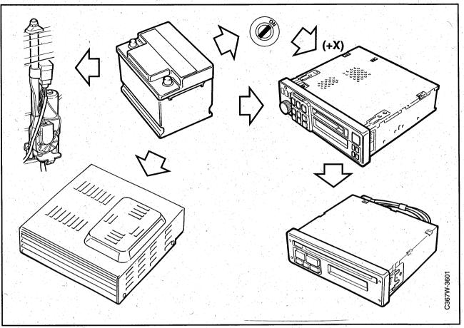
The radio and cassette unit, amplifier and the power antenna are supplied with +30 via fuse 19.
