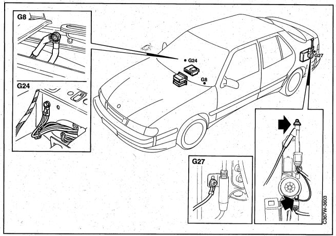
The radio and cassette unit are grounded to grounding point G8.
