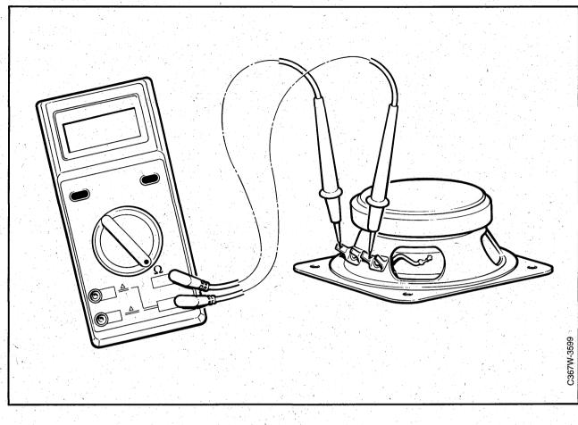
Coil resistance is measured between the speaker connector pins with connectors, filters and capacitors removed.
