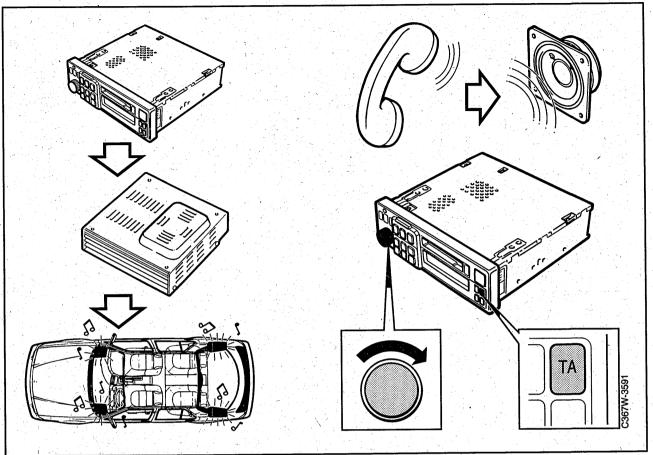
The audio signal is fed to the speakers from the amplifier located under the right-hand front seat.
