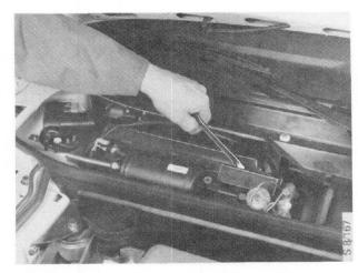
2 Unplug the connectors and remove the thermostat.
