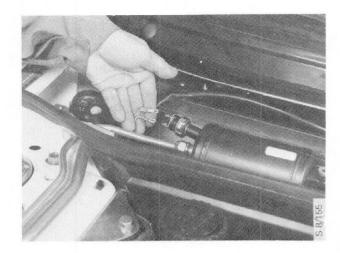
4 Pull away the rubber moulding a little and withdraw the pipe from the plastic lead-through. Disconnect the pipe coupling. Blank off the open ends.
