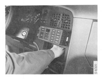
4 Remove the inside air sensor and unplug the connector.
