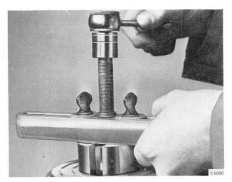
6 Remove the pulley assembly.
