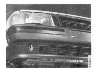
2 Undo the bumper securing bolts and lift off the bumper.
