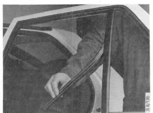
4 Undo the window channel screw and remove the channel.
