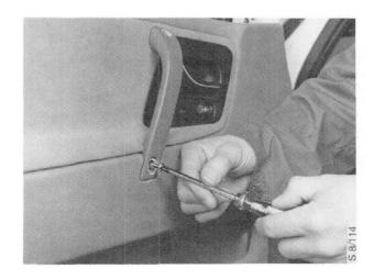
Twist the handle and pull free the lip at the bottom before removing.
