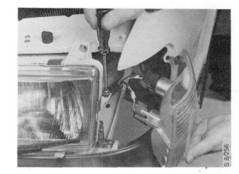
4 Undo the bolts securing the wing to the body and lift off the wing.
