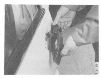
Lift off the handle. Separate the ball joint and remove it from the handle.
