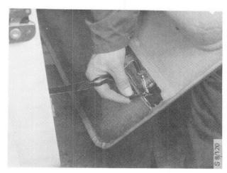
Cars with electrically adjusted door mirrors: disconnect the electrical connectors.
