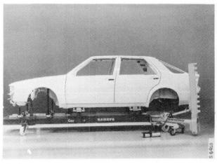
Body mounted on aligning bench
