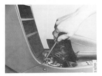
7 Remove the middle air vent on the panel.
