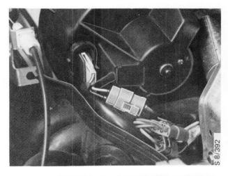
4 Disconnect the temperature control cable.
