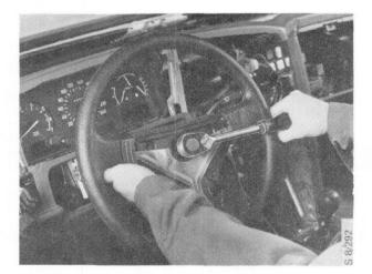
9 Remove the stalk switch unit. Mark the connectors to facilitate refitting.
