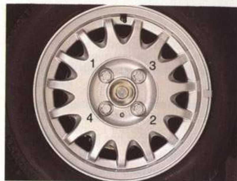
Tightening sequence for wheel studs
