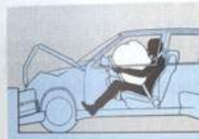
The airbag is completely inflated.
