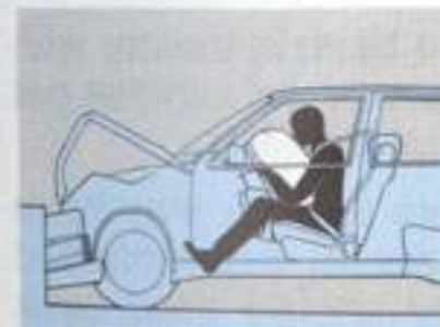
The steering column is crushed and the airbag starts to empty.
