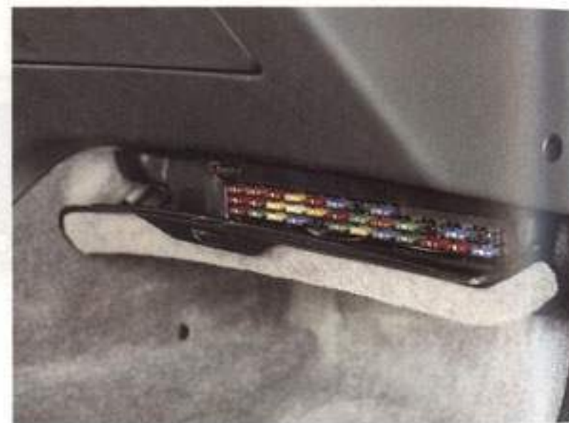
Main fuse box (cars with an airbag on the passenger side) SG1268
