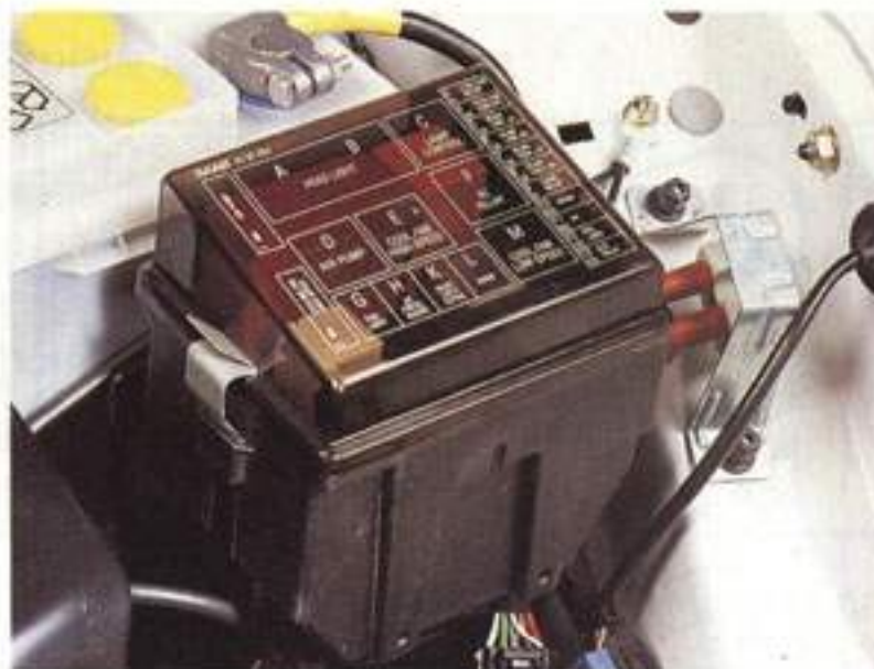
Power distribution panel in engine compartment SG1301
