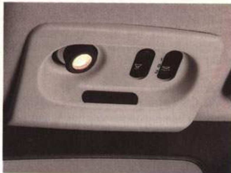
Switch for interior lighting
