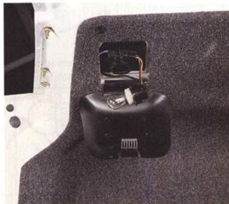
Changing bulb for rear fog light (9000 CD)
