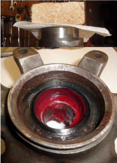
New seal and bearing loaded with grease, ready for installation.
