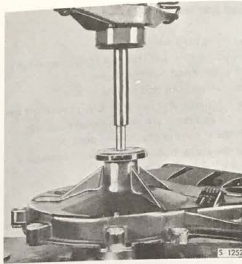
REMOVAL OF FAN BEARING Tool 78 62 436 and drift
