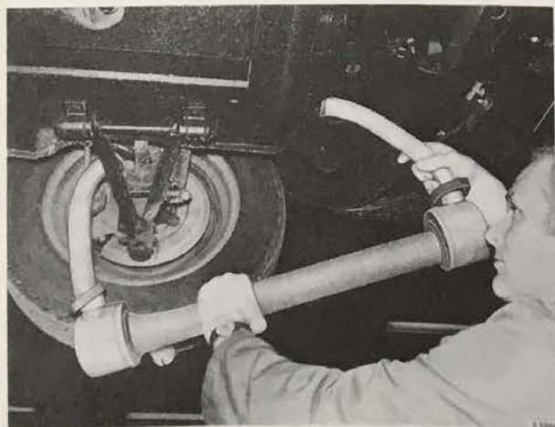
LEFT-HAND PIPE IS REMOVED THROUGH THE HOLE IN THE FLOOR
