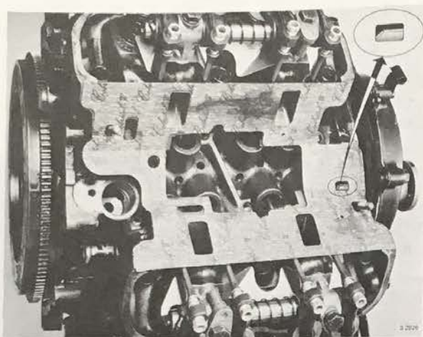
INSTALLATION OF INDUCTION MANIFOLD GASKET
