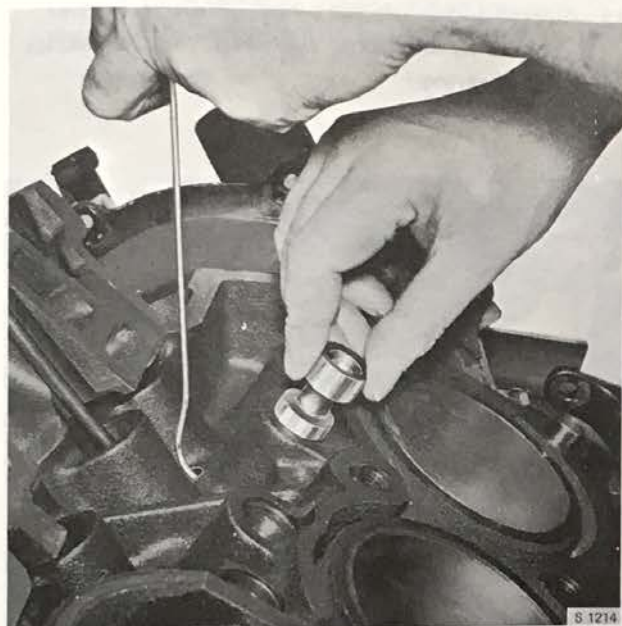
REMOVAL OF TAPPETS BY MEANS OF A BENT WIRE
