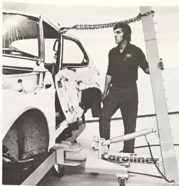
EXTENSION PIECE MOUNTED TO DRAW-ALIGNER ARM FOR THE APPLICATION OF LOADS AT ROOF HEIGHT
