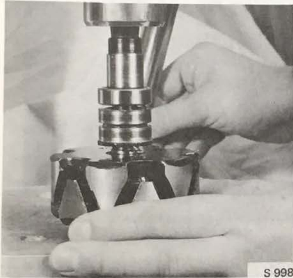
PRESSING IN THE SLIP RING END BEARINGS
