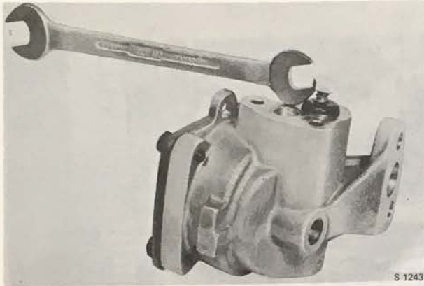
REMOVAL OF RELIEF VALVE COVER PLATE
