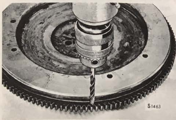
SPLITTING OF RING GEAR BY DRILLING
