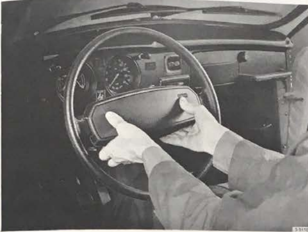
THE SAFETY PADDING IS REMOVED
