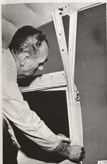
INSTALLATION OF DOOR PILLAR TRIM
