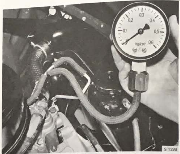
MEASURING FUEL PRESSURE
