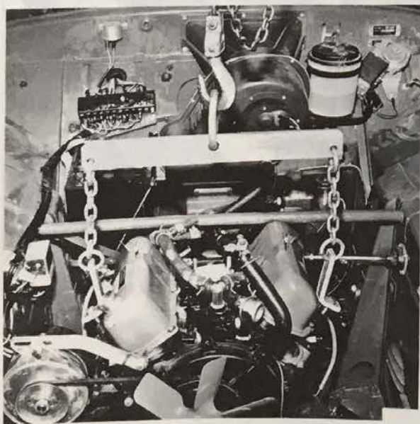
REMOVAL AND INSTALLATION OF ENGINE WITH LIFTING HOOK 78 62 022
