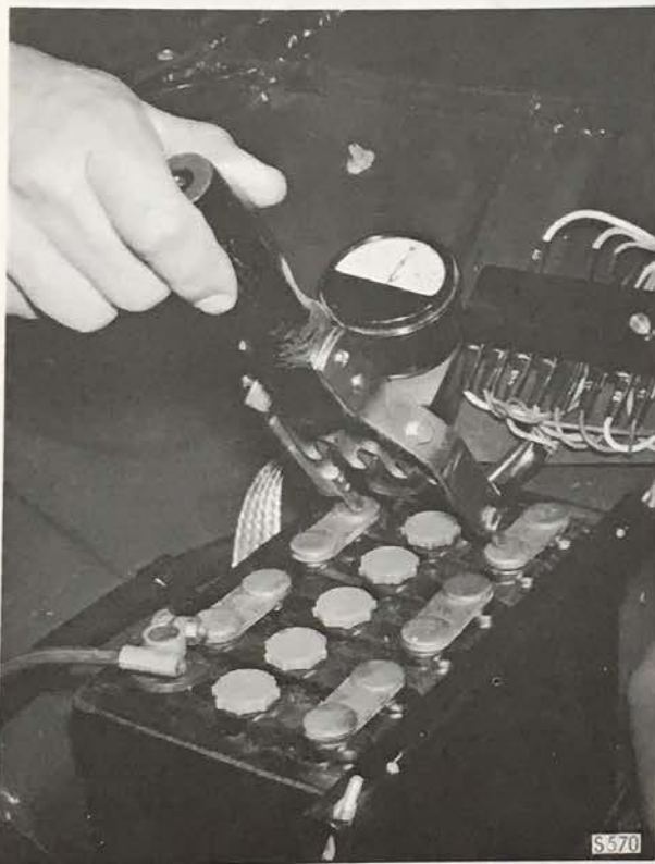
CHECKING THE BATTERY WITH A CELL TESTER
