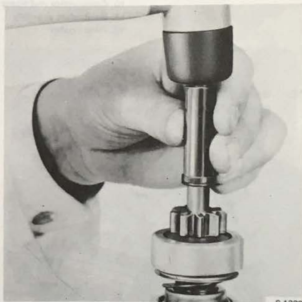
PRESSING DOWN THE STOP RING
