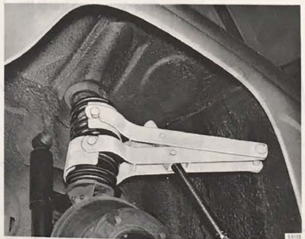
THE POSITION OF THE SPRING SCISSORS AND THE SPRING CUPS ON THE LEFT SIDE
