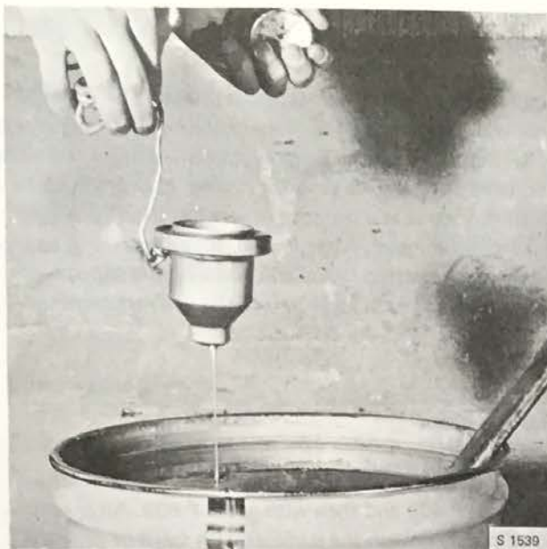
MEASURING VISCOSITY WITH AN SIS BEAKER
