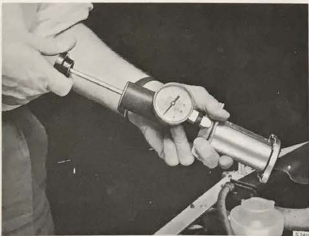
CHECKING THE OPENING PRESSURE OF THE PRESSURE CAP
