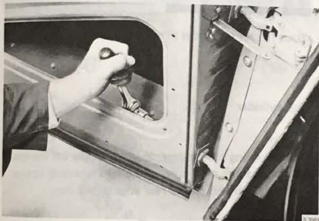
REMOVAL OF DOOR
