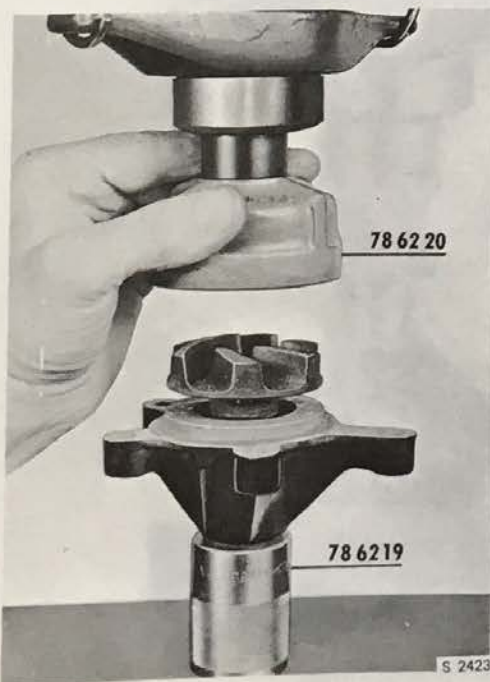
FITTING OF IMPELLER Tools 78 62 196 and 78 62 204
