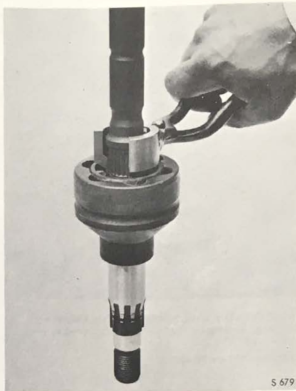
INSTALLATION OF INNER DRIVE SHAFT Tool 78 41 612
