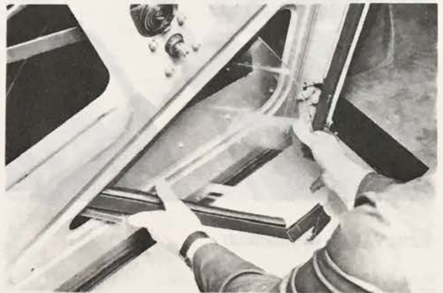
REMOVAL OF DOOR WINDOW
