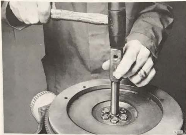
REMOVING THE DISC SHAFT BUSHING Tool 78 40 648
