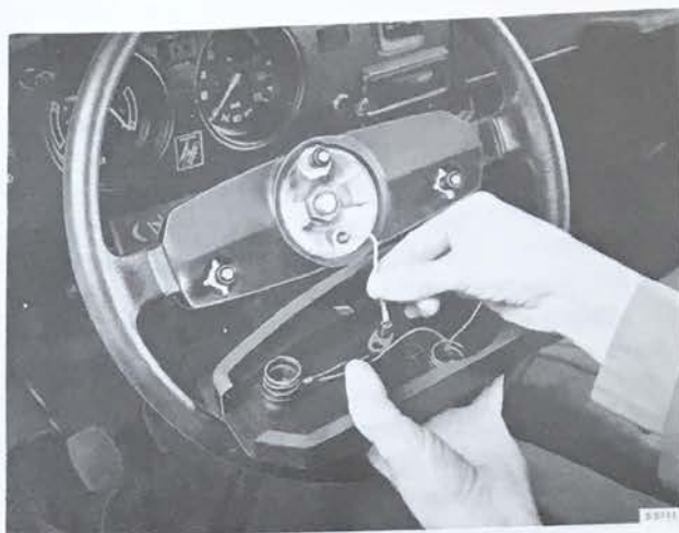
DISCONNECTING THE ELECTRIC CONNECTION
