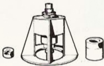
8392490 Installing and removing tool, water pump (earlier design)
