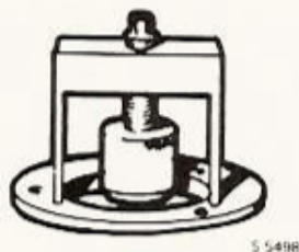
8392649 Installing and removing tool, water pump (later design)
