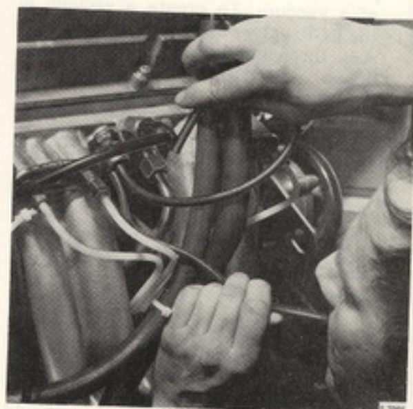
2. Clean the inlet and outlet of the EGR valve using a rotary wire brush. Take care not to damage the valve spindle when cleaning the outlet side. 3. Rinse the valve in trichloroethylene and blow the valve clean with compressed air, keeping it open by means of a wire.
