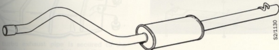
Rear pipe section
